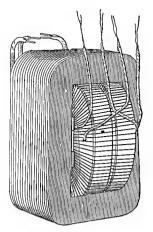
FIG. 95. View of shell-type (Fort Wayne Elec. Co., Type A) transformer.
